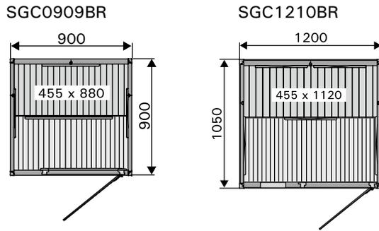
The wood material in Radiant infrared cabins is hemlock. The outer surface is dark walnut veneer. Walls, ceiling, floor, benches and backrests are pre-fabricated. Radiator elements are integrated into walls and benches. The floor is an integral part of the cabin.
